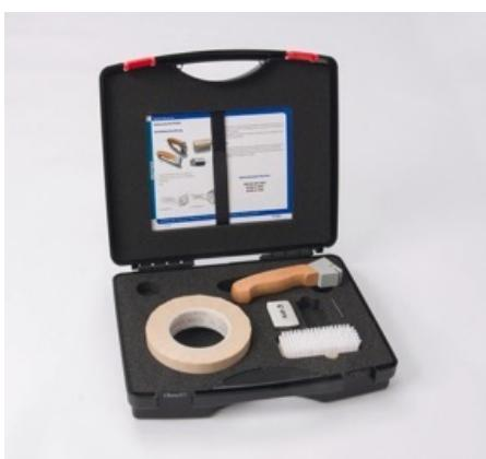
Determine the adhesion of coating onto different rigid surfaces.
