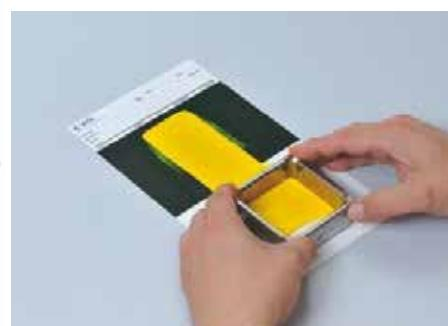
Application equipment that allows liquid coating to be applied from 25 – 1250 micron depending on the specific application.
