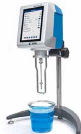
Viscosity measurements using a Byk-Gardner Rotational viscometer.
