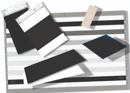
A range of standard test substrates for coating application performance testing.
