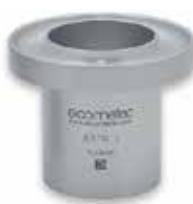
Flow cup measurements for lower viscosity/ Newtonian liquid samples.
